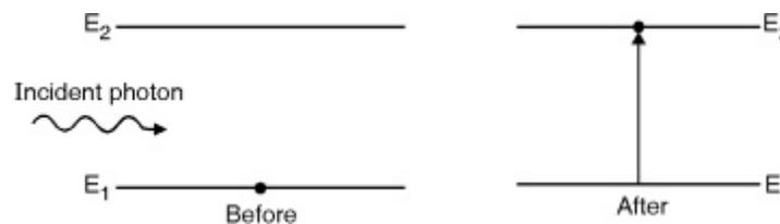
Fig. 4.2.1 : Induced absorption
